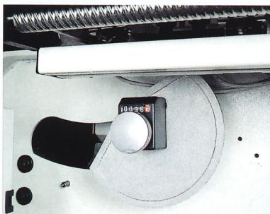
A patented system enables micrometric adjustment of scoring saw travel to match panel thickness.
