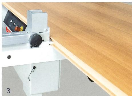
Referencing system for first trim cut with metric rule readout (2-3)
